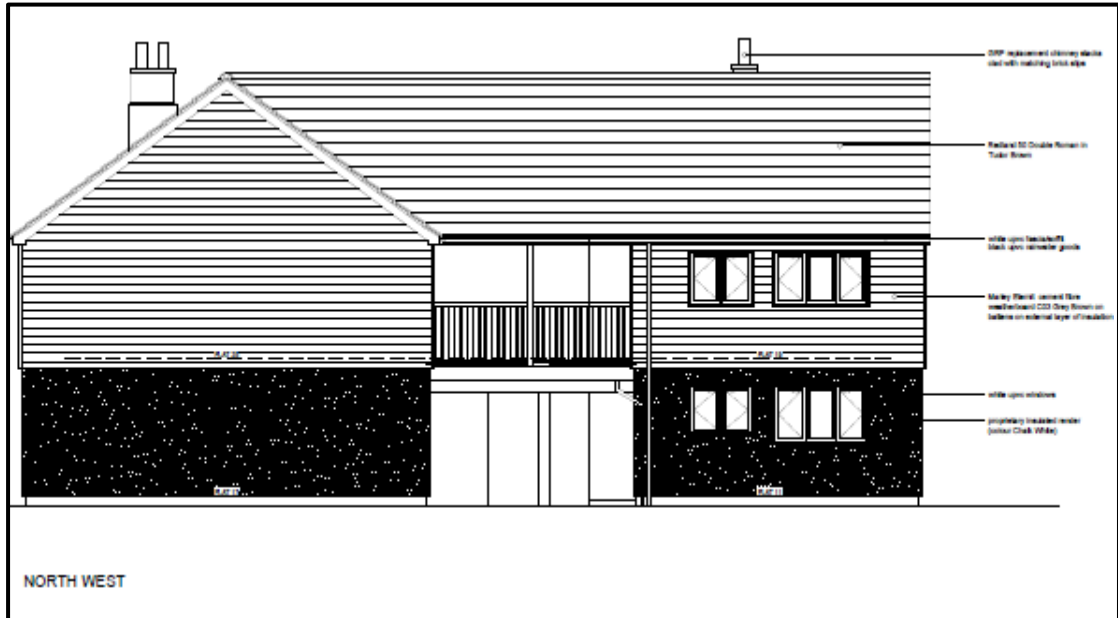
Figure 10 Proposed North West Elevation
